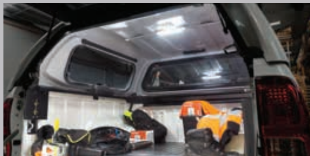
Example of one IONNIC Strip Light installed illuminating an entire canopy.
