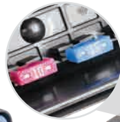
Holds 4 spare fuses inside of cover
