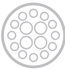
SG16 Cavity Configuration 12 x Ø 1.6mm Contacts 4 x Ø 3.5mm Contacts
