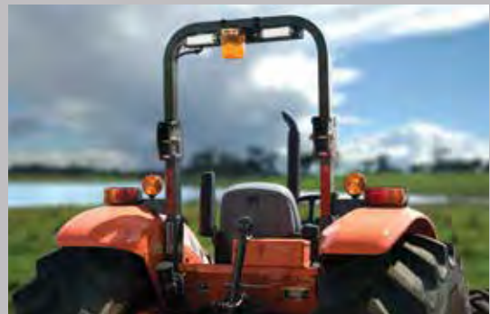
Typical Installation showing bar clamped to ROPS.
