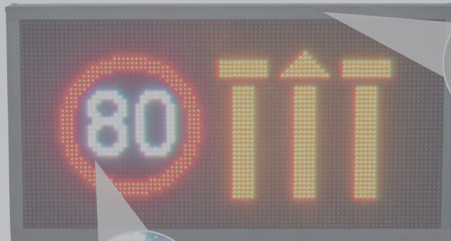
Each LED module contains a red, green & blue LED
