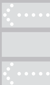
Flashing Arrow Left
