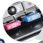
Holds 4 spare fuses inside of cover
